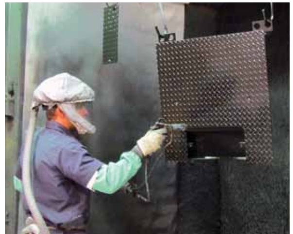
Carbon steel floor scales are given a protective coating of two-part epoxy paint.
