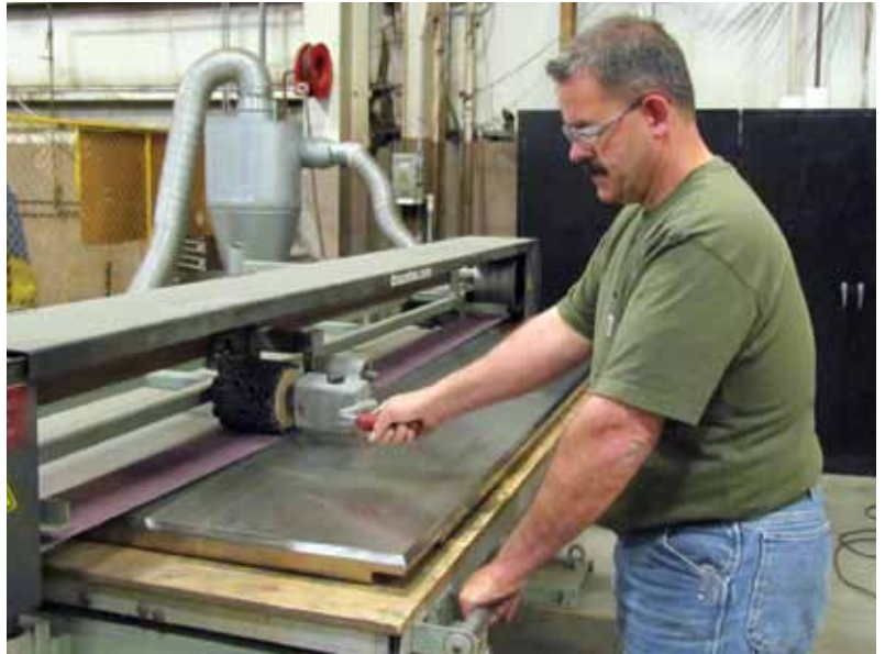
An in-house stroke belt sander is used for polishing floor scale platforms to meet the requirements of sanitary applications.
