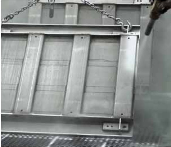
Our standard finish for stainless steel floor scales is provided by glass bead blasting.
