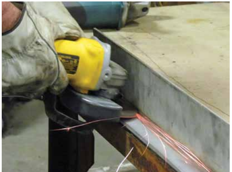
For sanitary applications, welds are ground smooth before a scale is polished.
